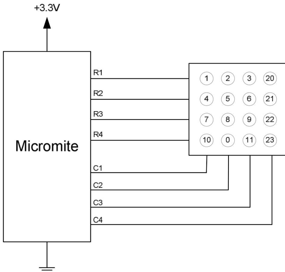
The detection and decoding of key presses is done in the background and the program will continue after this command without interruption. When a key press is detected the value of the variable var will be set to the number representing the key (this is the number inside the circles in the diagram above). Then the interrupt will be called.
