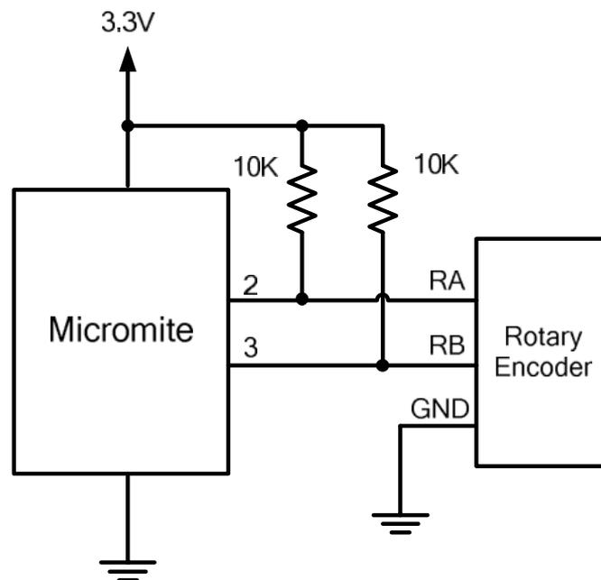
And this program fragment can be used to decode the output:
