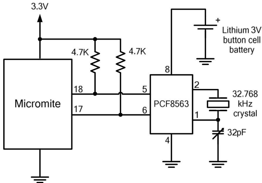
The 32pF adjustable capacitor should be used to trim the crystal frequency for very accurate timekeeping but that can be tedious as it will involve checking the time for drift over days and weeks. If you don't want to do that you can substitute a 10pF capacitor or leave it out completely and the timekeeping will still be reasonably accurate.
