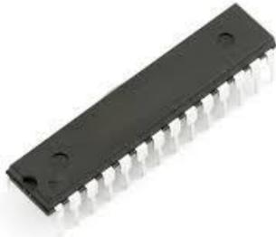
The Micromite is a Microchip PIC32MX150/250 series microcontroller programmed with the MMBasic firmware. This chip is available in a low cost 28 pin dual in line package which can be easily soldered and plugged into an IC socket.
