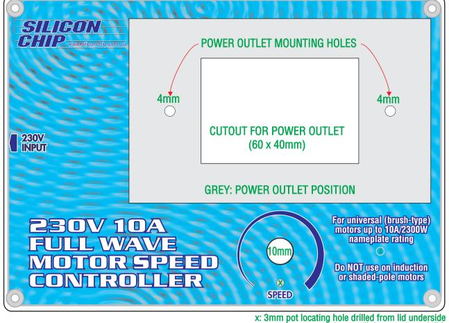
x: 3mm pot locating hole drilled from lid underside - does not need to go all the way through lid.
