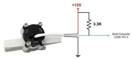
If you use a paddle wheel flow sensor you must check the specifications and only use one that specifically states that it is suitable for use with petrol or diesel fuel. RS Components have a suitable sensor (part nbr 508-2704) and <u>www.lightflying.com.au</u> or <u>oregonlightsport.com</u> have a similar sensor made by MGL Avionics.
