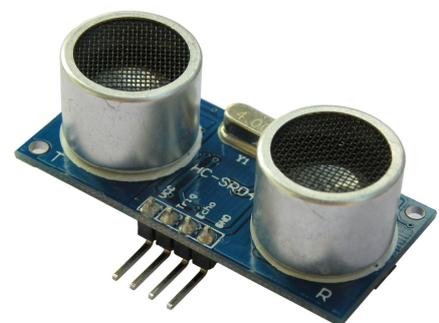
The I/O pins are automatically configured by this function but note that they should be 5V capable as the HC-SR04 is a 5V device. You can use multiple sensors connected to different I/O pins or even sharing the one trigger pin if care is taken to prevent one sensor from interfering with another.
